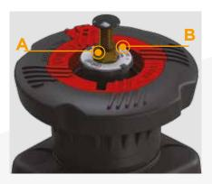
**Travel stop adjustment** To set the lock to the minimum flow rate or closed position, rotate the handwheel until the required position is reached and then lock the set position by tightening nut (A) and locknut (B).
